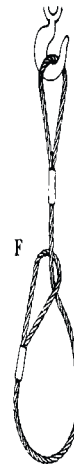
Fig. 7f. Choker Hitch One leg vertical, with slip-through loop Rated capacity is 75% of the single rope in Fig. 7a.
